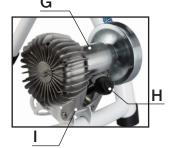
**8.** Before proceeding make sure that the rear tire of the bike is properly inflated. Check the sidewall of the tire for the manufacturer's recommended pressure range, and inflate accordingly. Using the Adjustment Knob "H" set the Fluid Resistance Unit "I" so that the roller contacts the bike's rear tire. Then turn the Adjustment Knob "H" clockwise two full turns to insure that you have sufficient pressure of the Drive Roller "G" on the rear tire.
