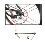
2. Replace the quick-release skewer on the rear wheel of your bike with the Quick-Release Skewer "K" included with the trainer. This assures ideal clamp fitting and stability.
