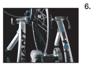
6. Place the bike's hub (outside width of Quick-Release Skewer) between the Couplings "B" and adjust the Coupling Knob "D" until the bike's rear tire is centered on the Drive Roller "G" of the Fluid Resistance Unit, then lock the hub by pressing down the Quick Release Lever "A" - the Quick Release Lever should be able to close without excessive force, and without visibly deforming the trainer's frame.
