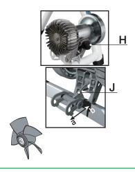
**3.** The Linkage pillar **"J"** is controlled by the Wheel Adjustment Knob "H". Try to move linkage pillar from frame attachment stay tracking location (a) to (b) until it's locked.
